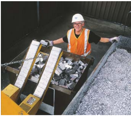
Compressed blocks of swarf ready for recycling. Energy required for off-site re-smelting is reduced because the density of the brick has been increased, and greenhouse gas emissions are also reduced because coolant has been removed.
